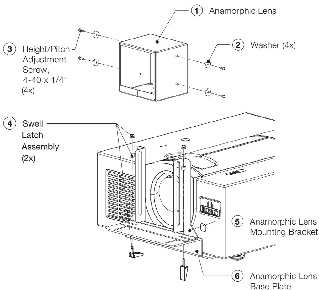
**Figure 3-17. Anamorphic Lens Mounting Assembly - Exploded View**
