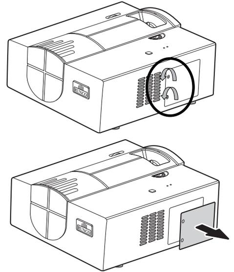
4. Loosen the four lamp assembly mounting screws.
