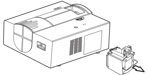
6. Gently slide the new lamp assembly into the mounting frame. Align the two power connectors at the top of the lamp assembly with the two sockets at the top of the mounting frame. Press gently on both sides of the lamp assembly to snap it into place. As you do so, the lamp cooling interlock switch returns to the ON position.
