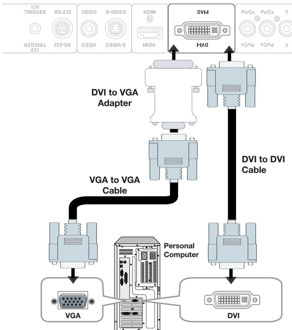
**Figure 3-10. RGB Connections**
