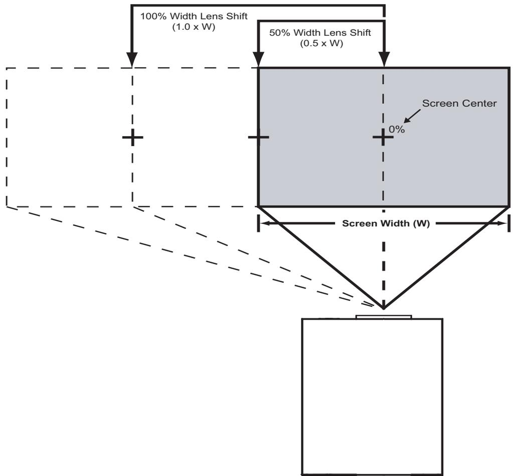
**Note:** This is a general example of lens shift. Lenses vary in their shift capabilities. **No particular lens or projector is shown in this example.**
