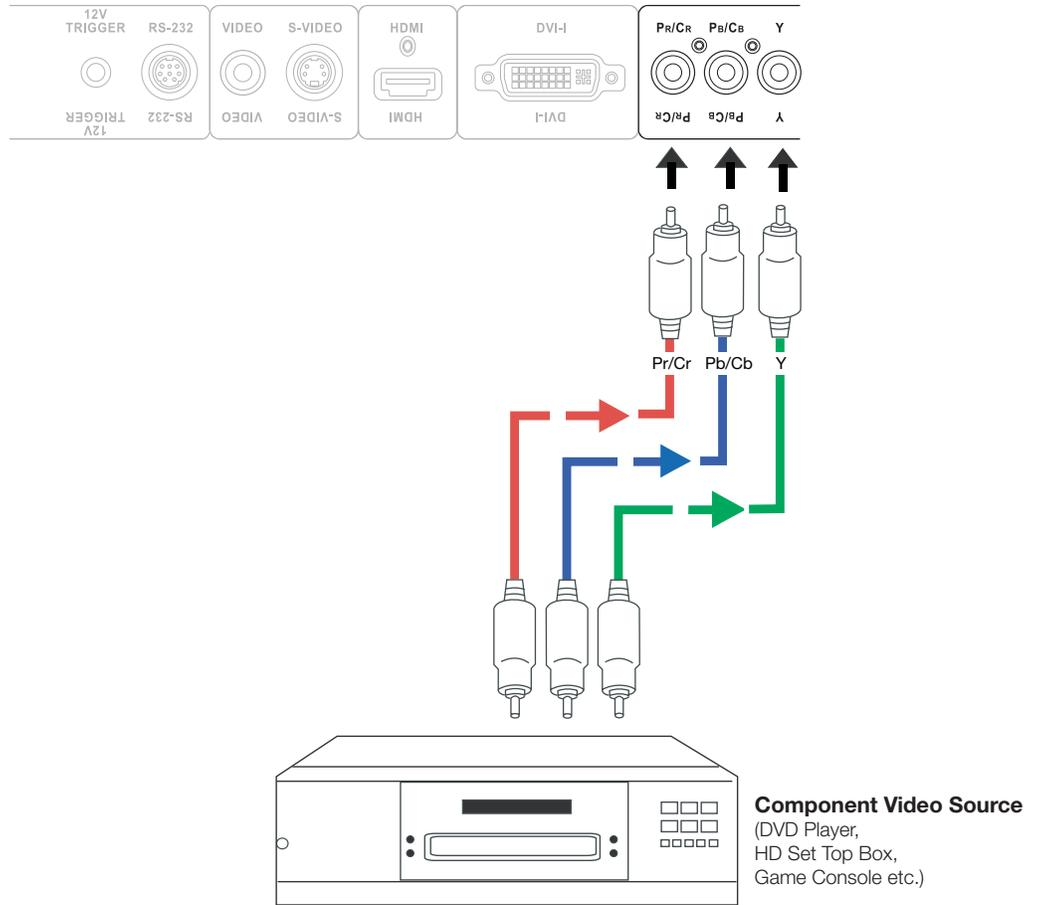
**Figure 3-11. Component Video Connections**
