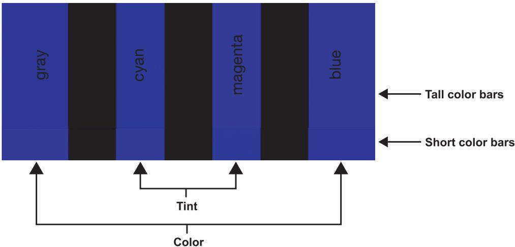
**Tint:** Tint or “hue” is essentially the ratio of red to green in the color portion of the image. When tint is decreased, the image appears redder; when it is increased the image appears greener. To set the tint, select Tint from the Adjustment menu and press **ENTER**. While looking at the color bar pattern through a blue filter, adjust the tint level until the cyan and magenta color bars (on either side of the green bar) appear to be a single shade of blue.
