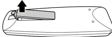
2. Insert the included batteries. Ensure that the polarities correctly match the ⊕ and ⊖ markings inside the battery compartment.
